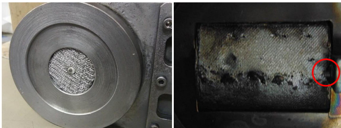
Figure 2. Left: Investigated target (circular center region) consisting on a W felt substrate covered by Sn with a LP tip embedded at the center before exposure to particle beam heat fluxes. Right: Studied SnLi target (after its exposure to particle beam and laser heat fluxes) presenting a LP lateral configuration (tip visible within red circle)
