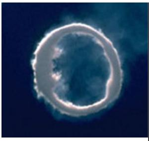
The Outer Mode was identified in JET as a low  $n$  ideal external kink, driven by the edge density.
